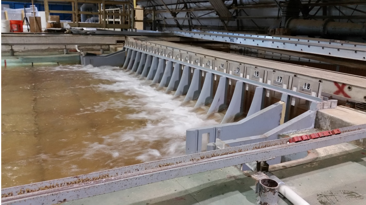
Photo 2 Bonneville Spillway 1:55 Model
