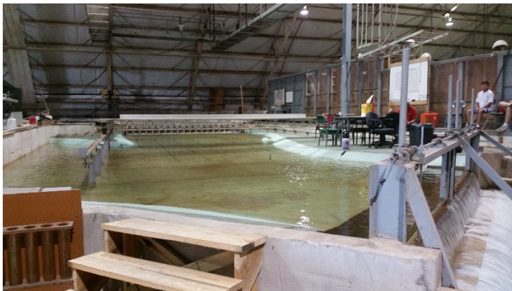
Photo 1 – Bonneville 1:55 Spillway Model
